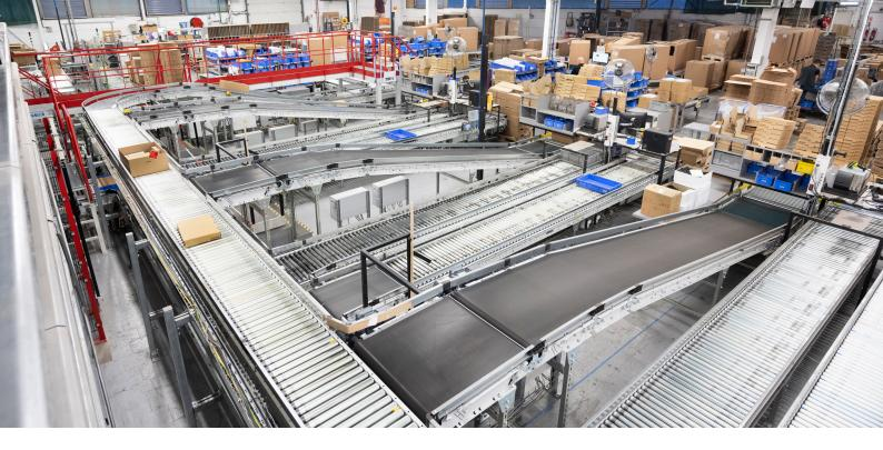
Within the multishuttle system, 12 shuttle vehicles take over the order sequence formation. The conveyor technology transports the requested articles to the various workstations. Thus, the intralogistics solution has completely automated the previously manual storage and retrieval as well as order picking of the goods and the entire material flow.
